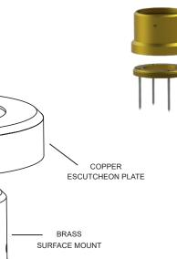
CONCRETE ANCHOR SCREWS (INCLUDED) **SM-BD400 Heavy Duty Surface Mount** (120V) Machined from solid brass the Surface Mount is equipped with stainless steel hardware and a unobtrusive spun copper escutcheon to hide mount screws. For durable installations of up to 48" high bollards mounted to solid, level surfaces only. Designed to fit over up to three 3/4" bundled PVC conduits.
