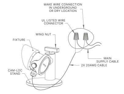
**Important!** This fixture is assembled and sealed at the factory, do not unscrew any of the pre-assembled caps or the cord seal. Doing so could result in leakage and failure.
