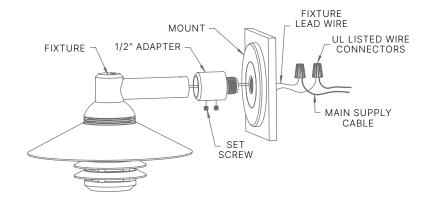
TIP: Small gauge cable is vulnerable to damage in the landscape; Protect by routing in close proximity to the luminaire or adjacent to concrete slab or similar structure. Do not over tighten.
