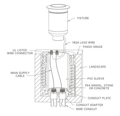
**TIP:** Small gauge cable is vulnerable to damage in the landscape; Protect by routing in close proximity to the luminaire or adjacent to concrete slab or similar structure. Do not over tighten.
