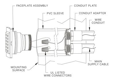
**TIP:** Small gauge cable is vulnerable to damage in the landscape; Protect by routing in close proximity to the luminaire or adjacent to concrete slab or similar structure. Do not over tighten.
