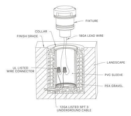
TIP: Small gauge cable is vulnerable to damage in the landscape; Protect by routing in close proximity to the luminaire or adjacent to concrete slab or similar structure. Do not over tighten.
