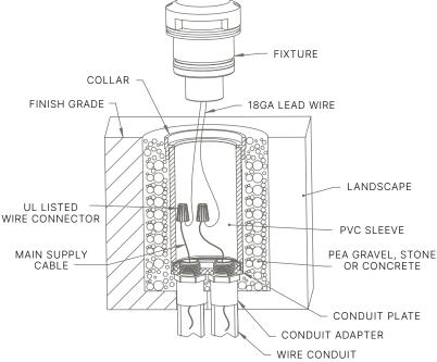
**TIP:** Small gauge cable is vulnerable to damage in the landscape; Protect by routing in close proximity to the luminaire or adjacent to concrete slab or similar structure. Do not over tighten.
