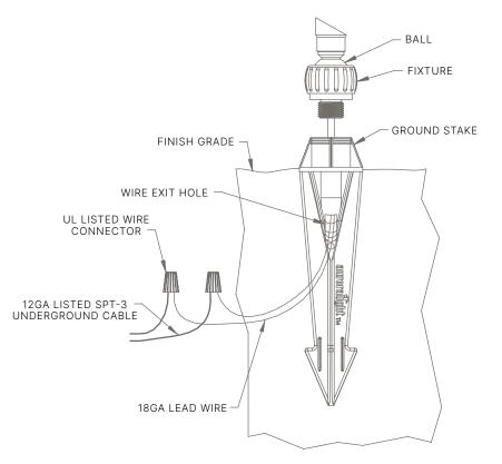
**TIP:** Small gauge cable is vulnerable to damage in the landscape; Protect by routing in close proximity to the luminaire or adjacent to concrete slab or similar structure. Do not bury more than 6" deep. Do not over tighten.
