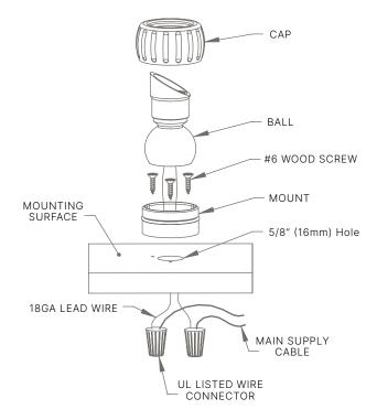
**TIP:** Small gauge cable is vulnerable to damage in the landscape; Protect by routing in close proximity to the luminaire or adjacent to concrete slab or similar structure. Do not bury more than 6" deep. Do not over tighten.
