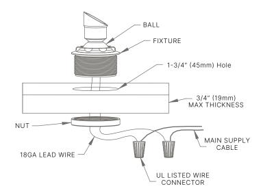
**TIP:** Small gauge cable is vulnerable to damage in the landscape; Protect by routing in close proximity to the luminaire or adjacent to concrete slab or similar
