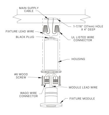
**TIP:** Small gauge cable is vulnerable to damage in the landscape; Protect by routing in close proximity to the luminaire or adjacent to concrete slab or similar structure. Do not bury more than 6" deep. Do not over tighten.
