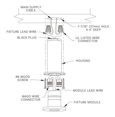
**TIP:** Small gauge cable is vulnerable to damage in the landscape; Protect by routing in close proximity to the luminaire or adjacent to concrete slab or similar structure. Do not bury more than 6" deep. Do not over tighten.
