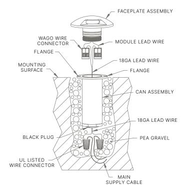
**TIP:** Small gauge cable is vulnerable to damage in the landscape; Protect by routing in close proximity to the luminaire or adjacent to concrete slab or similar structure. Do not over tighten.
