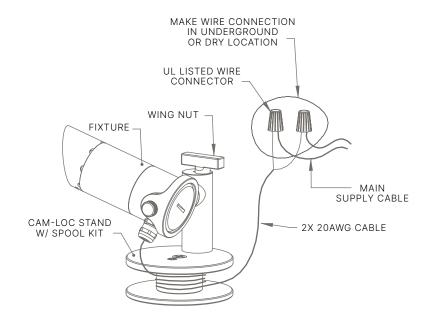
**Important!** This fixture is assembled and sealed at the factory, do not unscrew any of the pre-assembled caps or the cord seal. Doing so could result in leakage and failure.
