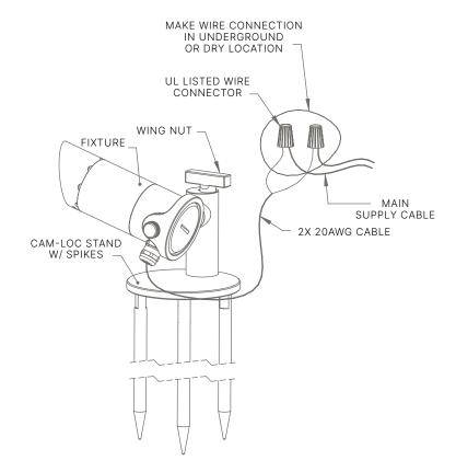
**Important!** This fixture is assembled and sealed at the factory, do not unscrew any of the pre-assembled caps or the cord seal. Doing so could result in leakage and failure.
