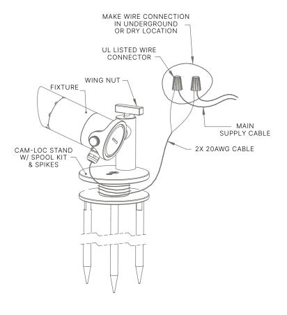
Important! This fixture is assembled and sealed at the factory, do not unscrew any of the pre-assembled caps or the cord seal. Doing so could result in leakage and failure.
